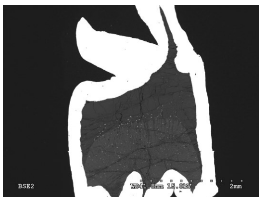
Figure 2: Example of a black shale melting experiment performed at 850°C. The product consists of about 50% melt (top part of capsule) and 50% residual crystals (lower part of the capsule)
