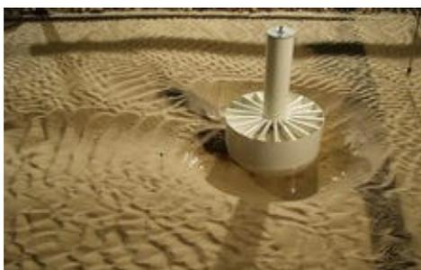
One of the models Richard uses to study scour around wind turbine foundations
