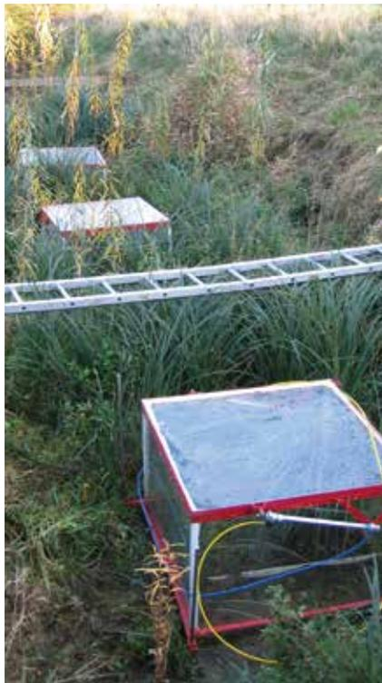
Automated chambers at work measuring nitrous oxide emissions from a farm drainage ditch.
