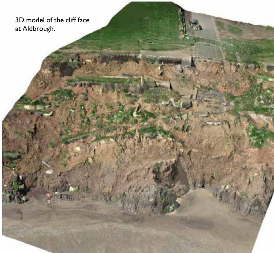
UAVs are helping NERC's British Geological Survey (BGS) understand and monitor areas that are susceptible to landslides around the UK, allowing the authorities to manage risks to the public more effectively. BGS researchers use a range of UAVs including a six-rotor model known as the Hexakopter, which flies slowly around the landslide, taking many overlapping photos from different angles. They then use a computer to stitch these images together into a 3D model of the cliff face.
