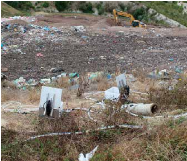
Automatic flux chambers on the slope of a hill of capped refuse.
