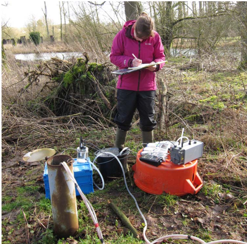
Monitoring of methane in groundwater
