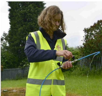
Figure 1. Collecting a groundwater sample for dissolved methane analysis.
