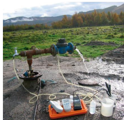
Figure 2. Measuring groundwater chemistry at a newly drilled well.
